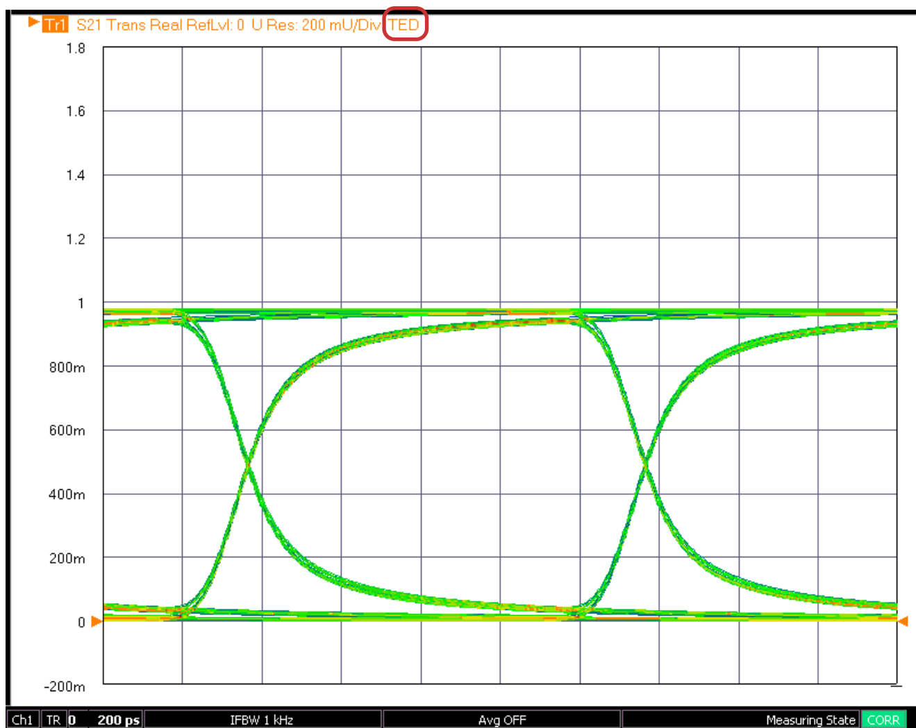
Figure 25-18. Time, Eye Diagram Display Example – Note that when in Time, Eye Diagram mode, the display trace annotation displays “TED”.
